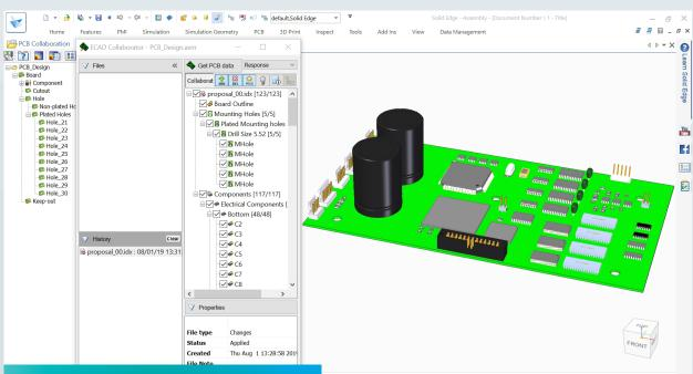
Solid Edge PCB Collaboration enables users to import precise models, providing a true 3D view of the design, one that can be rotated and visually inspected for interferences.
