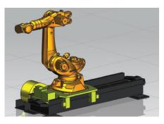
Six- and seven-axis robotic configurations can be defined and used in NX, including robots on rails and work positioners.
