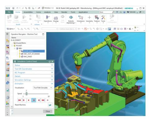
With NX CAM Robotics Programming, you can easily create cutting, trimming or grinding motions and simulate the robot as it performs the role of the machine tool.
